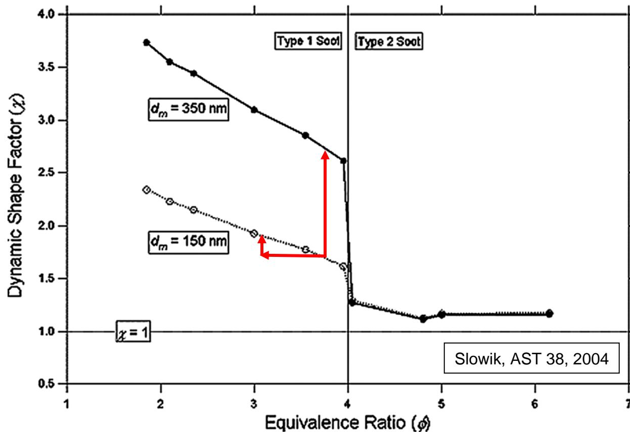
$$\phi = \text{fuel}/\text{O}_2 \text{ (actual)} / \text{fuel}/\text{O}_2 \text{ (stoichiometric)}$$
