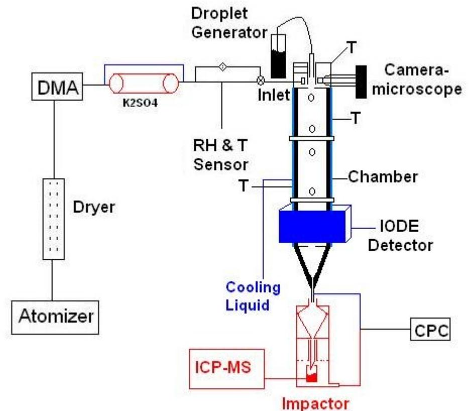
Collision efficiency experiment (CE)
