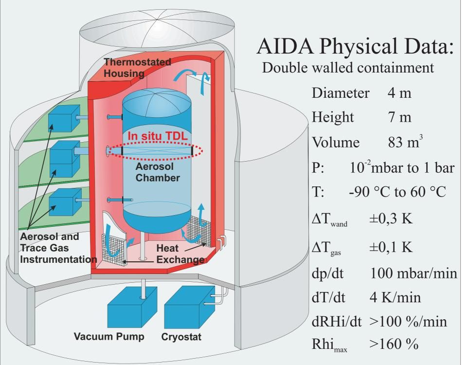
Temperature stabilized and ice covered inner reactor wall
