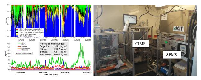
Examples of single particle fractions (upper panel, SPMS) and particle mass concentrations (lower panel, AMS) and view into the measurement container with 3 mass spectrometers.
